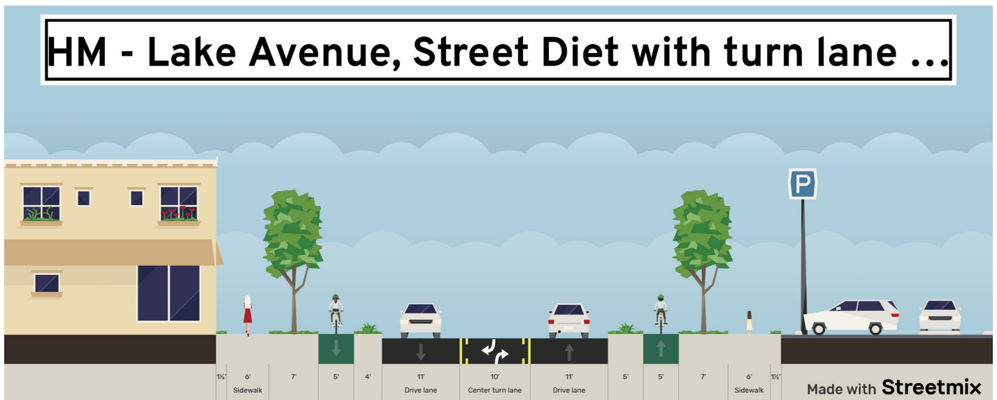
Typical Section of Lake Ave with sidewalk level bikeways and center two way turn lane
