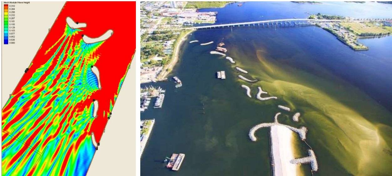
Computer Sediment Modeling and Aerial Photo of Sediment Transmission on Site
